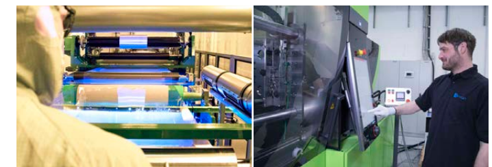
UV- rollimprint (R2R) for lab-on-a-chip production
