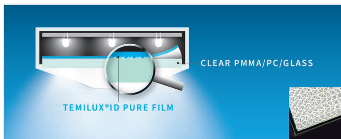
temiLux®ID pure film with microstructures facing away from LEDs (inside)
